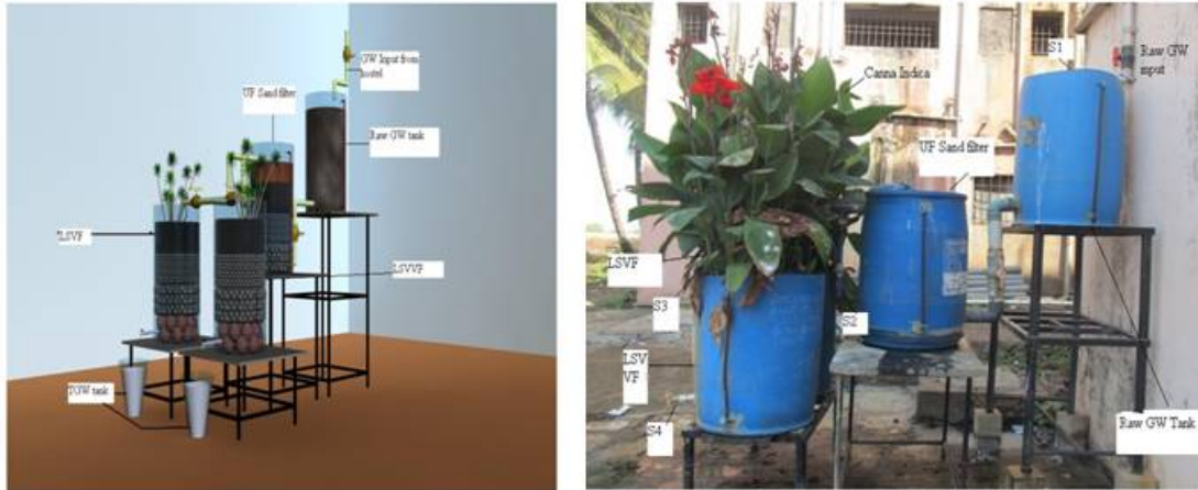
Figure 1: Schematic Diagram of Laterite Soil Vegetated Vermifilter a) Side View b) Front View
