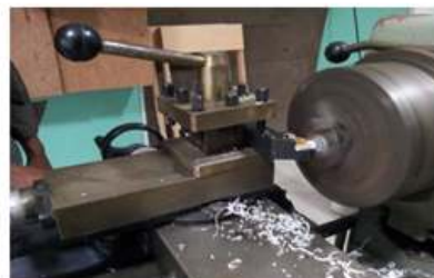
Figure II.5.b.: Cut acrylic stub shaped into a cylinder using a lathe machine
