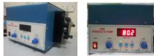
Figure II.2.a: Pulsatile flow inducing pump i) Oblique view of Peristaltic pump ii) Front panel of the pump
