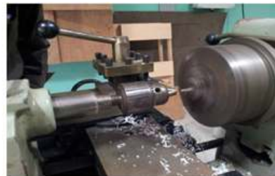
Figure II.5.c.: The acrylic cylinder drilled coaxially using lathe machine
