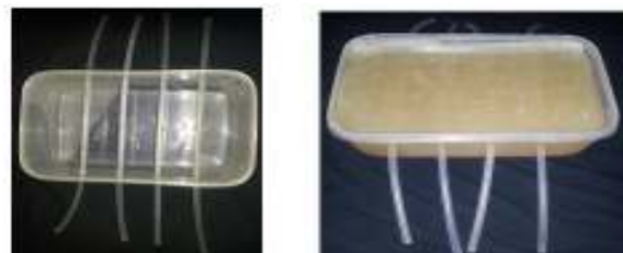
Figure II.6.c.: Tissue and Tube phantom container i) EVA tubes inserted through the drilled holes of the Plastic container ii) Agar-Gelatin mixture filled into the container and layered with gelatin to mimic skin
