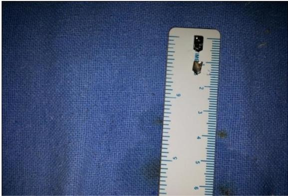
**Figure 1:** The broken blades of the flipcutter
